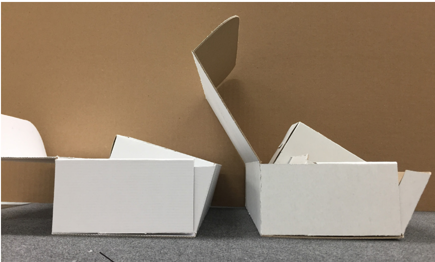
INITIAL CANTILEVER METHOD DID NOT ACHIEVE ENOUGH HEIGHT
