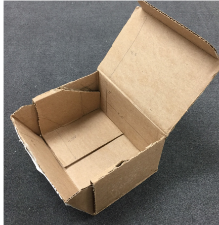
DOUBLE DOOR OPENING REJECTED FOR SHIPPING CONCERNS
